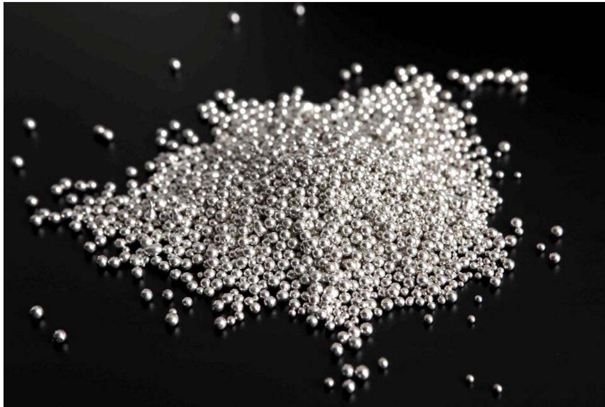
Indium pearls (photo by courtesy of Umicore Precious Metals Refining)
